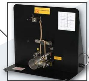
F300C - Experimental Impulse Turbine Module
