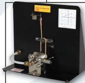
F300D - Experimental Reaction Turbine Module
