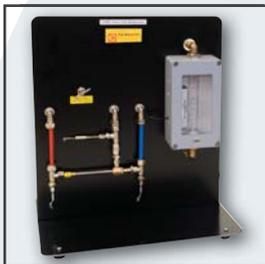
F300F - Vortex Tube Refrigerator Module
