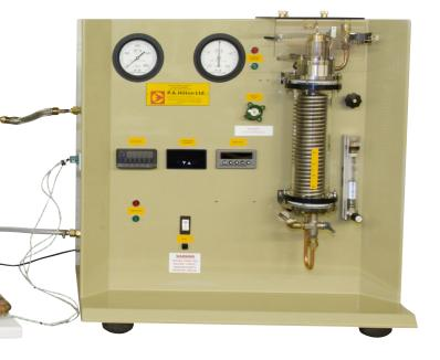
This is a closed loop unit supplied as two complimentary modules containing the certified electric boiler, pump, impulse turbine and condenser. The unit allows students to identify and compare theoretical maximum efficiencies with actual overall results.
